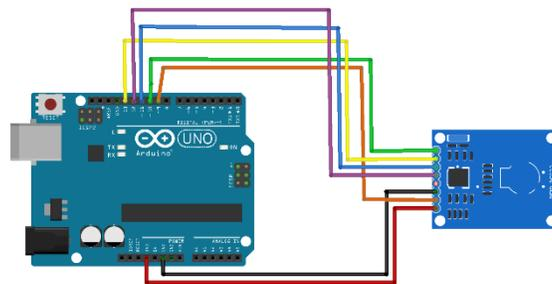
**Fig. 5:** Connection of the microcontroller with RFID module[26]
