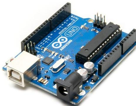
**Fig. 4:** Arduino Uno R3 Board [6]
