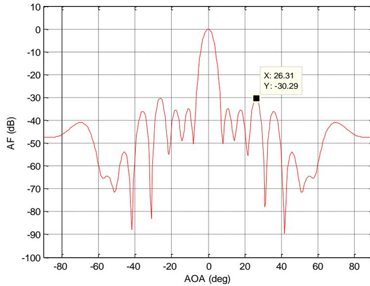
**Figure 5:** Radiation pattern for 18 Elements using GA
