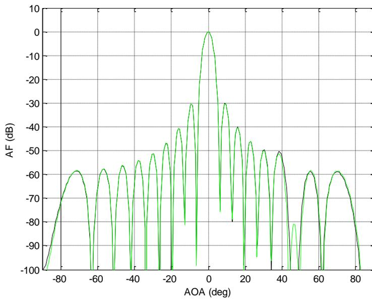
Figure 2: Radiation pattern for 18 Elements using LMS Algorithm
