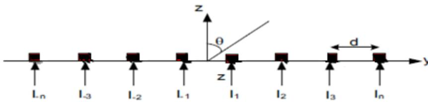
Figure 1: Equally Spaced Linear Array Arrangement [12]
