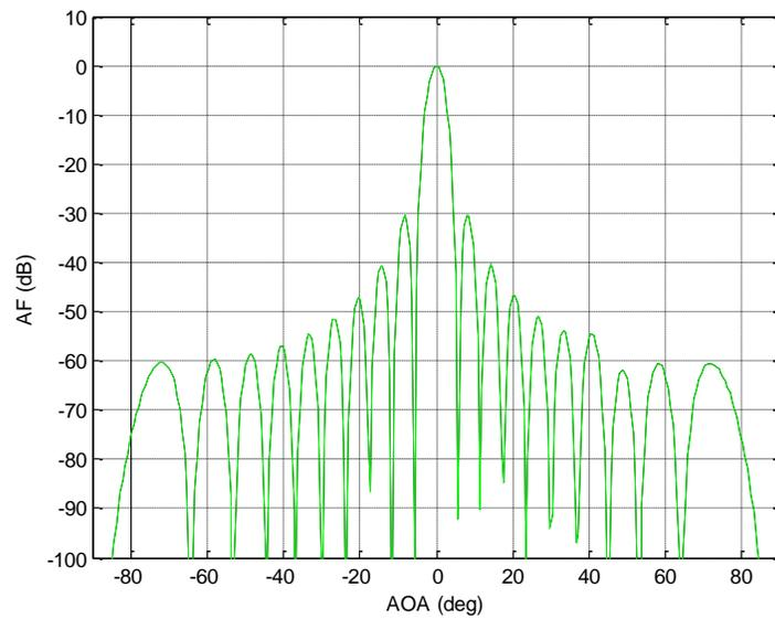
**Figure 4:** Radiation pattern for 20 Elements using LMS Algorithm
