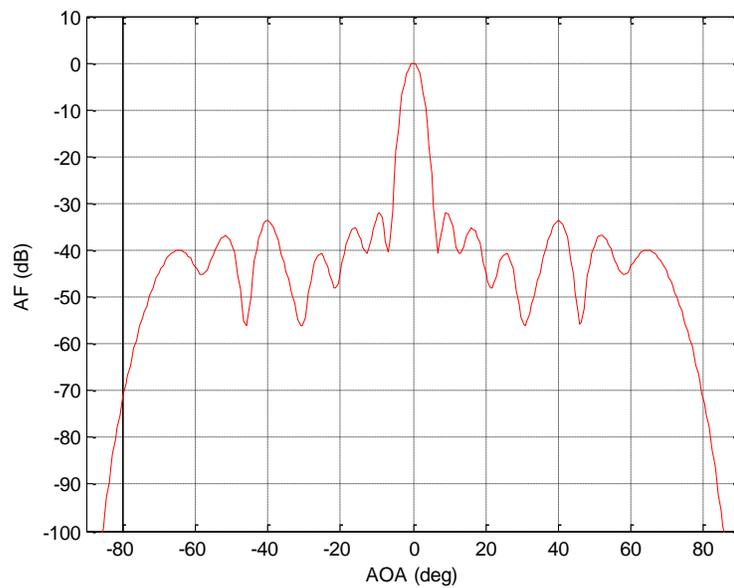
**Figure 6:** Radiation pattern for 20 Elements using GA
