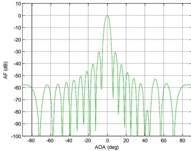
**Figure 3:** Radiation pattern for 19 Elements using LMS Algorithm
