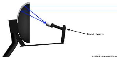
Fig. 4 The curved dish focuses incoming radio waves onto the feed horn.
