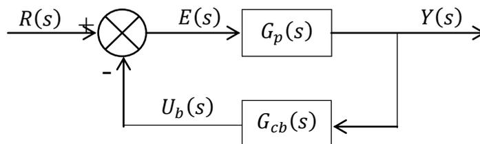
Figure 2: Block Diagram of Feedback Compensated System
