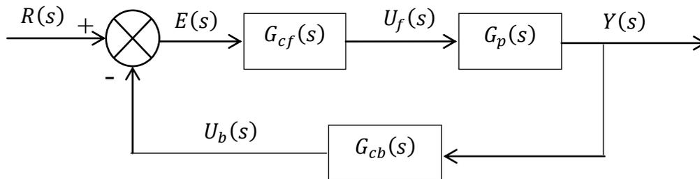
Figure 3: Block Diagram of Series-Feedback Compensated System
