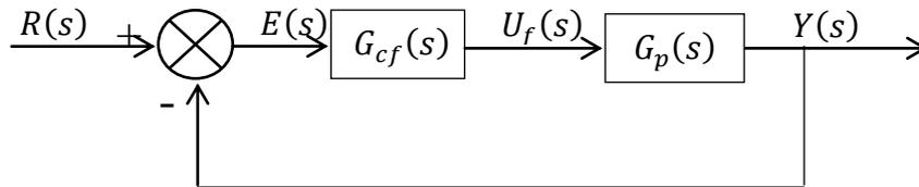
Figure 1: Block Diagram of Series Compensated System
