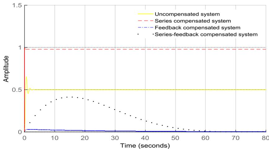
Figure 4: System Step Response before Tuning the Controller
