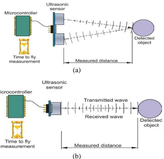
Fig. 2: The basic working principle of the ultrasonic sensor: (a). top view and (b). side view.
