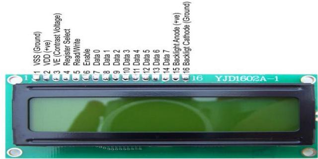
Fig. 5: The physical picture and pin definition of the YJD1602A-1 16-by-2 LCD display module.
