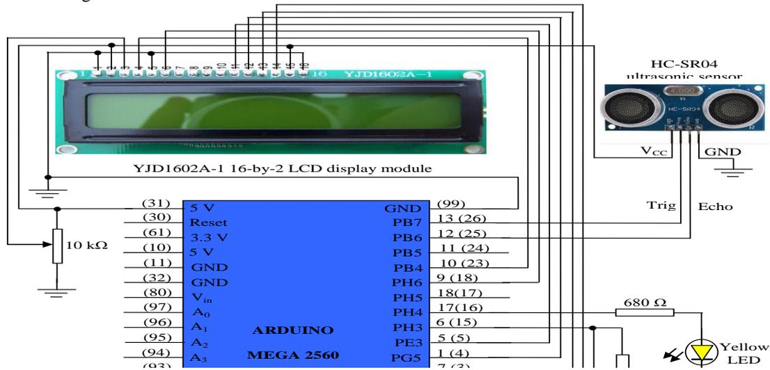
**Table 4:** Arduino Mega 2560 pin connections defined for the proposed EOD system design
