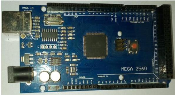
Fig. 4: The top view of Arduino Mega 2560 embedded development board.
