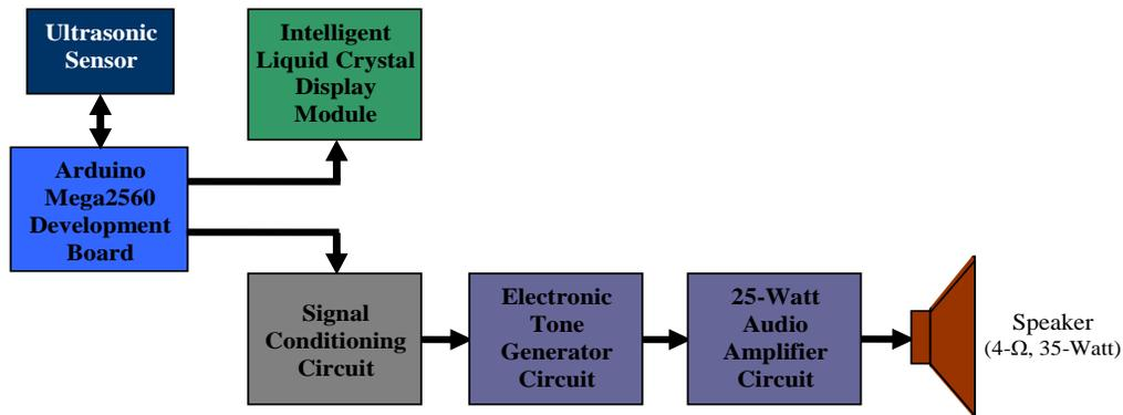
Fig. 1: The block diagram of the proposed enhanced obstacle detection system with alarm based on the Internet-of-Things (IoT).
