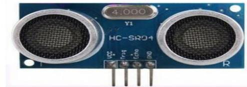
Fig. 3: The HC-SR04 ultrasonic sensors.
