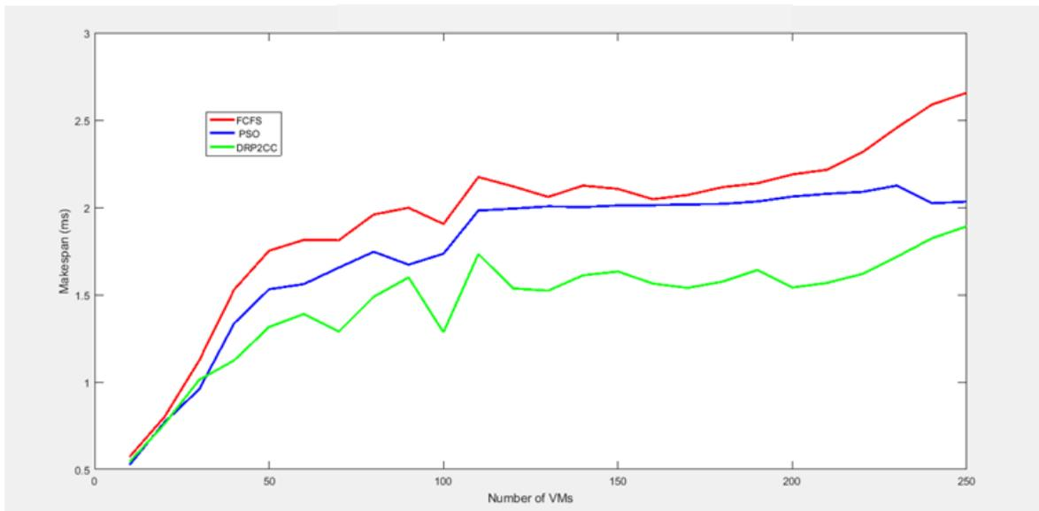
Fig. 3 Plot of makespan for DRP2C, PSO and FCFS.
