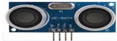
Fig. 3: The HC-SR04 ultrasonic sensors.
