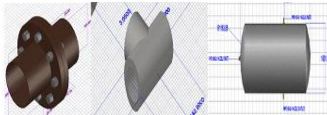
Figure 5: Flanges, Tee, and Storage Component Models (Source: [2])
