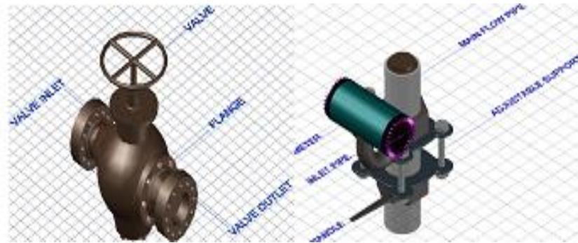
Figure 7: Valve and Flow Meter Models (Source: [2])
