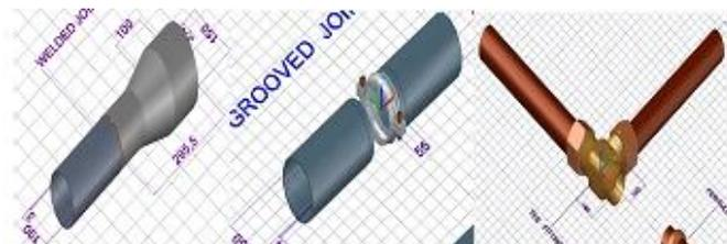
Figure 6: Pipeline Joint Models (Source: [2])
